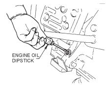
Figure 4. Engine Oil Dipstick
